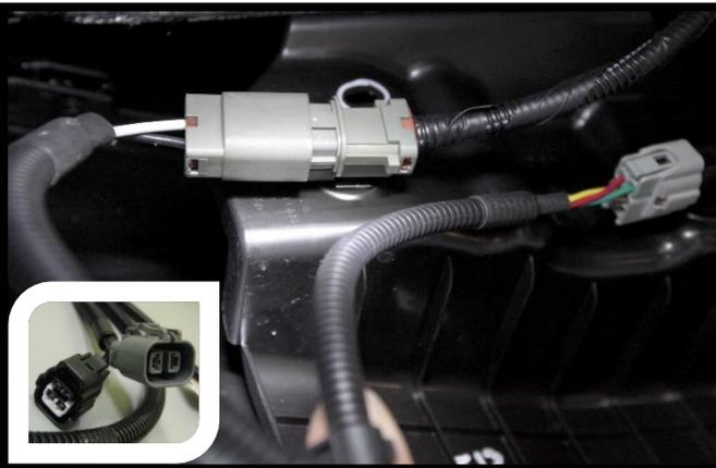
3. Plug in the trailer wiring harness's power line (2-pin) and signal line (4-pin) connectors to the corresponding connectors on the vehicle.
