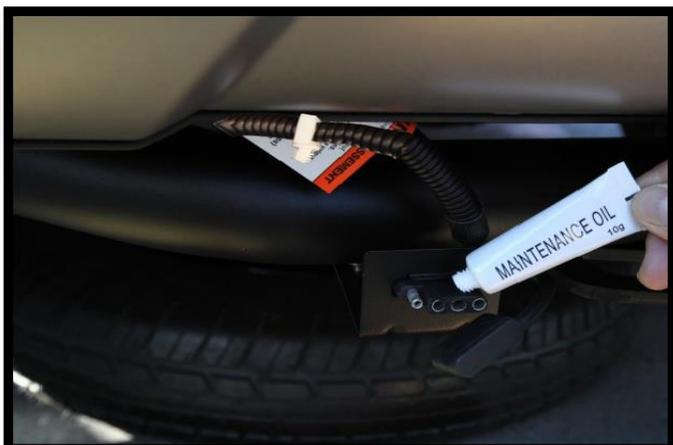
6. Insert the output connector (4-pin) into the wire holder on the hitch. Apply dielectric grease to the connector
