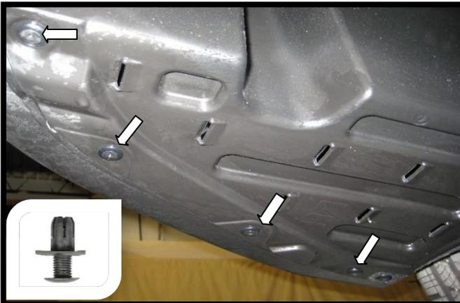
1. Remove 4 plastic retainers and then remove the driver side rear plastic undercover.
