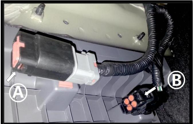
2. Remove the dummy protection connectors. Locking tab for connector A is located at the back. Locking tab for connector B is located at the top.
